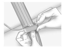
Place the guide over the belt and insert the two edges of the belt into the slots of the guide.
